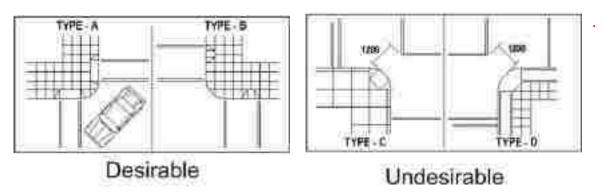
Figure 11-1: Kerb ramp placements at turnings
