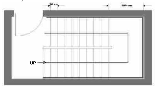
Figure 7-7: Continuous and extended handrail
