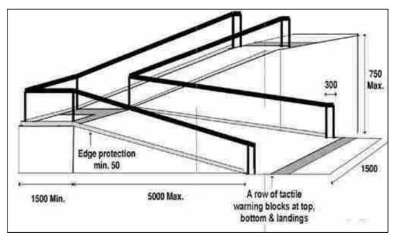
Figure 7-5: L-shape ramp with landing
