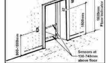
Figure 7-16: Layout of lift control panel
