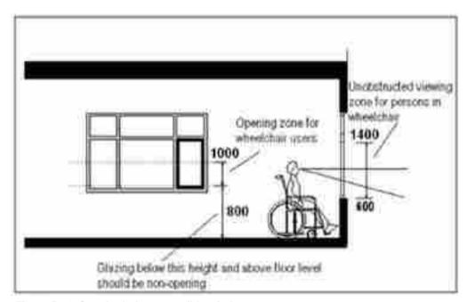
Figure 5-24: Standards for accessible window
