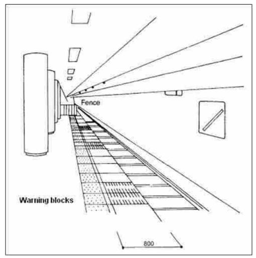
Figure 10-6: Warning blocks on platform edges
