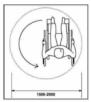
Figure 3-4: Turning radius
