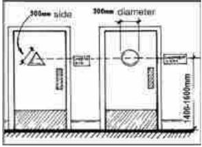
Figure 8-10: Placement of signage
