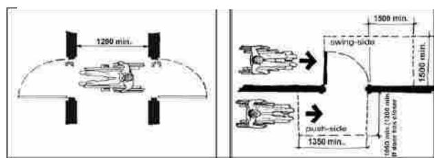
Figure 5-18: Maneuvering space needed for approach doors
