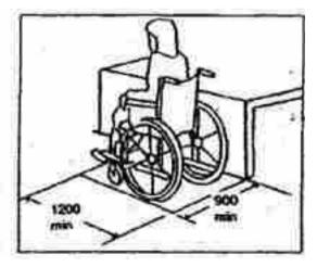
Figure 5-27: Space clearance for control operations
