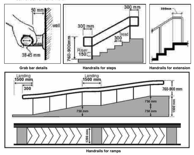
Figure 5-26: Handrail standards
