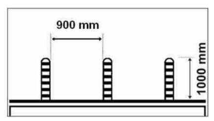
Figure 5-3: Bollards with spacing for wheelchair users/prams
