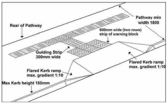
Figure 7-1: Kerb ramp detail
