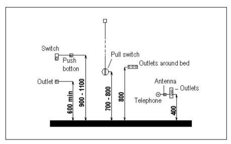
Figure 5-28: Location of electrical sockets, control, etc.
