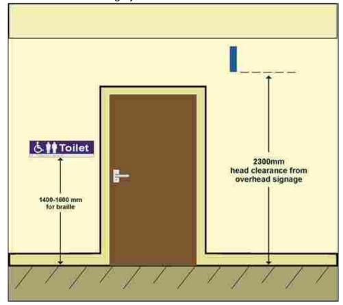
Figure 6-17: Height and placement of signages
