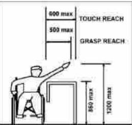
Figure 3-11: Forward and side reach over obstruction
