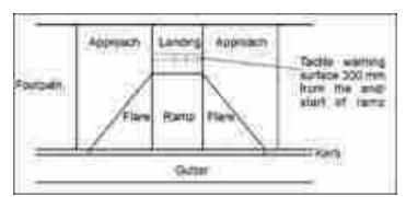
Figure 7-3: Typical kerb ramp requirements
